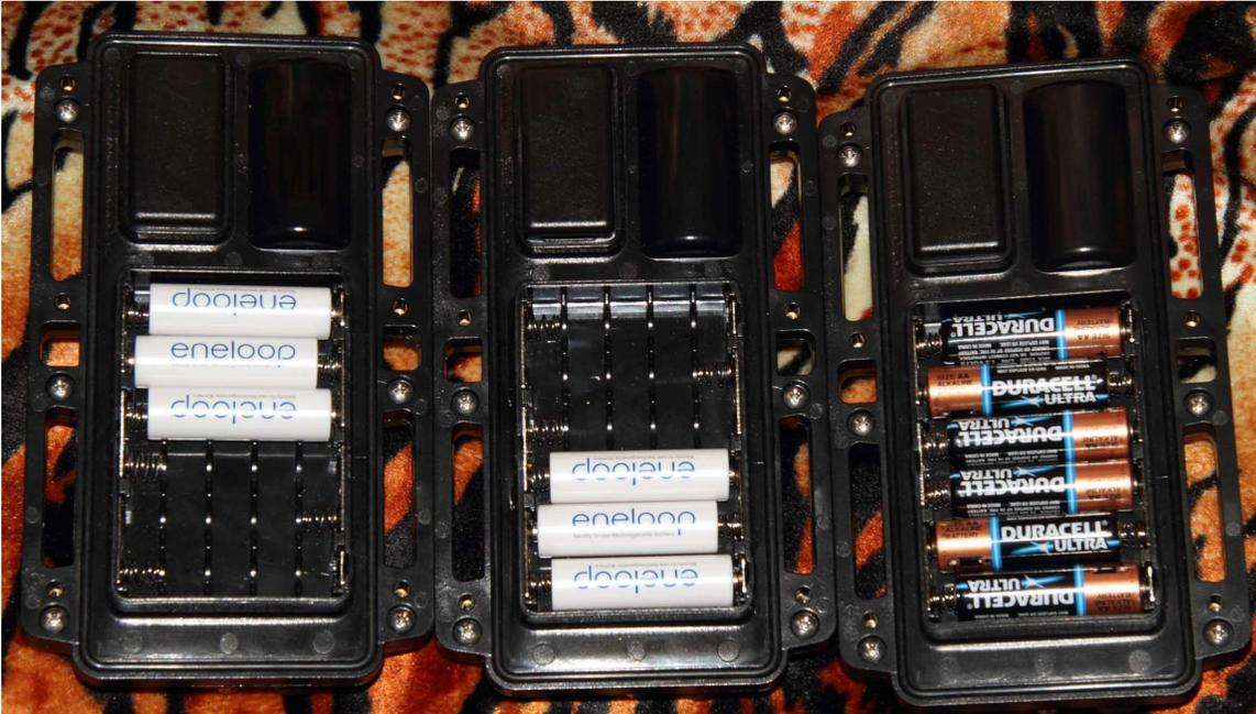
**Figure 2 - Battery compartment..** The battery compartment is accessed by removing the 6 screws on the back cover. The figure shows the three possible battery configurations that can be used. The batteries are arranged as two sets of 3 in parallel. The camera may be operated with 3 batteries in either of the two configurations on the left or with a full set of 6 batteries as shown on the right
